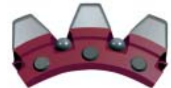
TYPE 4 Combined hardfacing of prepared grooves enhanced by two rows of tungsten carbide inserts
