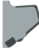
TYPE 4 Combined hardfacing of prepared grooves enhanced by two rows of tungsten carbide inserts
