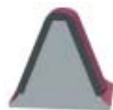
TYPE 3 Hardfacing is on all four edges and on the root face
