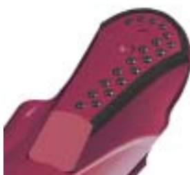
TYPE 4 Hard grain alloy is applied along the shirttail and leg leading edge. For additional protection tungsten carbide or diamond compacts are inserted on the leg of the bit.
