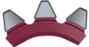
TYPE 2 Hardfacing of prepared grooves
