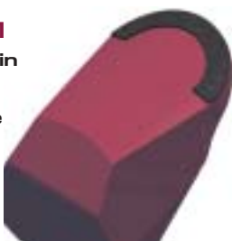
TYPE 4 Hard grain alloy is applied along the shirttail and leg leading edge. For additional protection tungsten carbide or diamond compacts are inserted on the leg of the bit.
