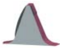
TYPE 2 Hardfacing is on the entering edge and on the origin of the trailing edge
