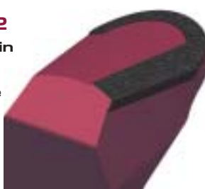
TYPE 5 Hard grain alloy is applied along the shirttail and leg leading edge. For additional protection tungsten carbide or diamond compacts are inserted on the leg of the bit. Stabilization pads containing carbide or diamond inserts are added to the bit leg to minimize wear and stabilize the bit in directional and horizontal applications.
